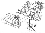
Fit the bar over the bar bolts. Place the bar in its rearmost position. Place the chain over the drive sprocket locate it in the groove on the bar. Begin on the top edge of the bar.
