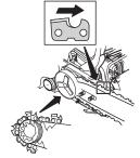
Make sure that the edges of the cutting links are facing forward on the top edge of the bar.
