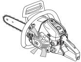
IMPORTANT! In order to maintain operation of the centrifugal cleaning system it must be regularly maintained. Clean the air intake to the starter, the fins on the flywheel, the space around the flywheel, inlet pipe and carburetor compartment.
