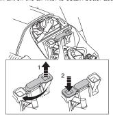
For temperatures below -5°C and/or in snow conditions a special cover is available, which is mounted on the starter housing.
